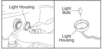
To replace the light bulb, pull the old light bulb out of the housing and insert a new light bulb. Re-attach the light housing to the spa shell. Re-attach the access panel to the spa.
